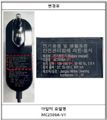
▲ Improvement of Defective Adapter Components and Specification Changes
